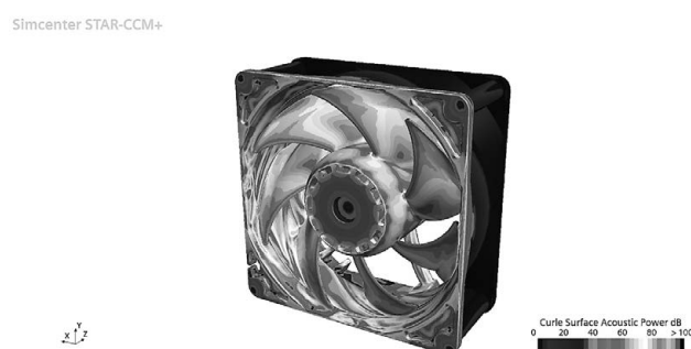
Fig. 6 Simulation-based sound source analysis example
